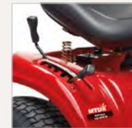
MANUAL CUTTING HEIGHT ADJUSTMENT AND MANUAL PTO
