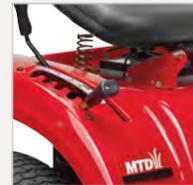
MANUAL CUTTING HEIGHT ADJUSTMENT AND MANUAL PTO
