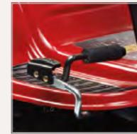
HYDROSTATIC TRANSMISSION ON ALL MODELS (HAND OR FOOT CONTROLLED)
