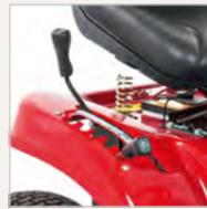
MANUAL CUTTING HEIGHT ADJUSTMENT AND MANUAL PTO
